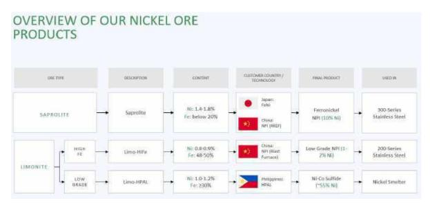
The Group ships out two (2) types of saprolite ore: high-grade and midgrade. High-grade saprolite has a nickel content of about 1.7% and above while mid-grade saprolite ore has a nickel content of between 1.3% to 1.6%.
